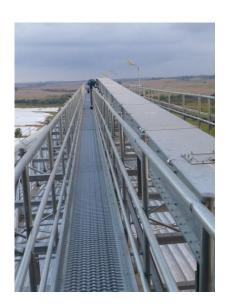
In 2012, we were contacted by a large grain producer overseas to create a solution for feed batching dryer systems with multiple inlets. The customer needed a conveyor capable of distributing material from one cell of the dryer to the next cell without opening or closing gates. The three cells had to be fed constantly and evenly. Sweet's solution was a horizontal conveyor with a double bottom.
